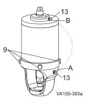
Figure 41 : Cap Screws and Vent Plug
