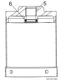
Figure 30 : Remove O-ring and Bearing
