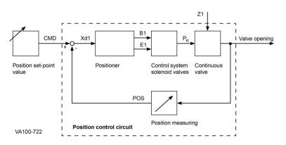
Figure 19 : Signal flow plan of position controller
