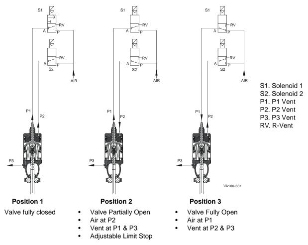
Figure 21 : 3-Position Actuator (AL) Function with External Solenoids
