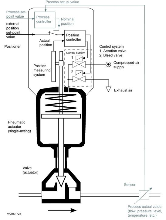
The black lines describe the function of the position controller (Type 8692). The gray lines illustrate functions typically performed by an external process controller or a more advanced control head (Type 8693).
