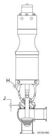
Figure 42 : Body to Adapter Gap
