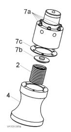
Figure 8 : Assembly of Range Spring and Components
