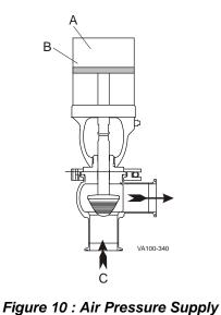
Product pressure up-stream or down-stream of the valve is controlled by changing the air pressure supplied to the actuator.
