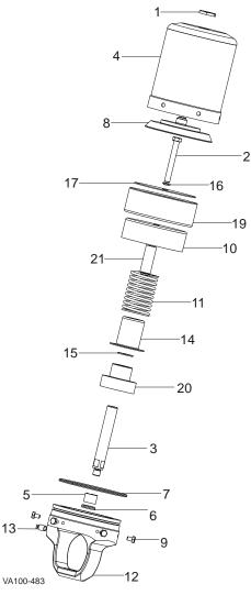
Figure 35 : 5" Air-to-Lower Diaphragm Actuator
