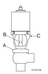
Removing Actuator/Stem Assembly from Valve Body
