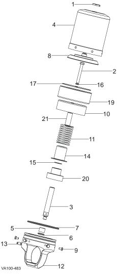
Figure 36 : 5" Air-to-Lower Diaphragm Actuator
