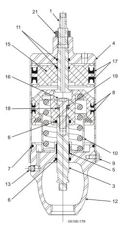
Figure 34 : 4" Air-to-Lower 3-Position Actuator
